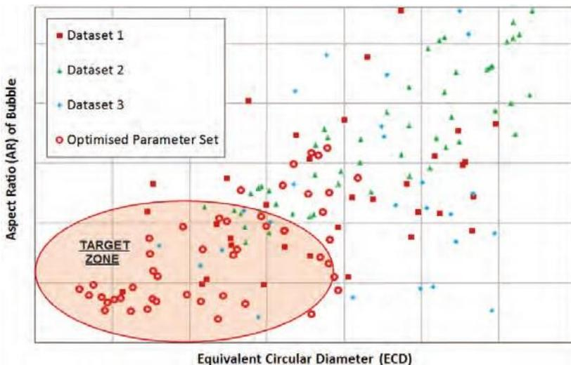
Bubble ECD and AR values obtained from optimized solution versus three previous bioreactor settings results.
