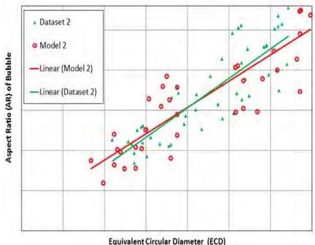
Comparison of bubble ECD & AR for COMSOL model versus physical test data obtained for two bioreactor settings
