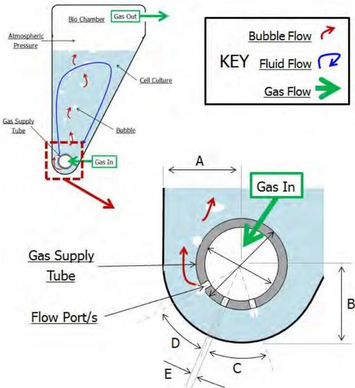
Schematic of section through bioreactor bag and parameters for assessment
